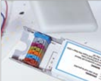
Philips Advance Xitanium LED drivers with SimpleSet technology have a designated blue area for contact with the programming device.
